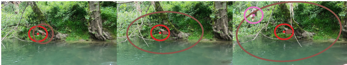
Figure 1: Our method : one object (red dot) is correctly detected at every frame and given a consistent identity throughout the sequence with low location uncertainty (red ellipse). Next to it, a false positive detection is generated at the first frame (brown dot) but immediately lost in the following frames: the associated uncertainty grows fast (brown ellipse). In our solution, this type of track will not be counted. A third correctly detected object (pink) appears in the third frame and begins a new track.
